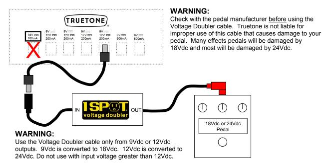
**NOTE**: Polarity for both input and output is center pin negative. If you have a pedal that requires center pin positive polarity, please use a Reverse Polarity Converter (CYR) or an L6 Converter (CL6), sold separately by Truetone. For example, old E-H Deluxe Memory Man pedals need a CL6 Converter, connected to the Output of the Voltage Doubler.
